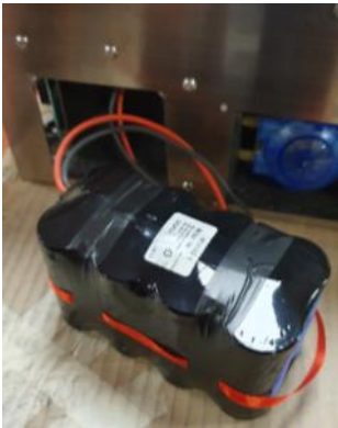
Figure 7 —System battery connector location.
