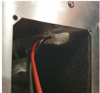
Figure 8 —Connect the battery connector to the charger.
